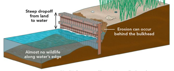
'Hard' infrastructure like retaining walls abruptly severs the ecological connection between the coast and water.
