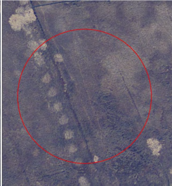
Example 2: Single ditch running through AA. 123.2 m 2 : 1.6% of AA is ditched: Score: 9
